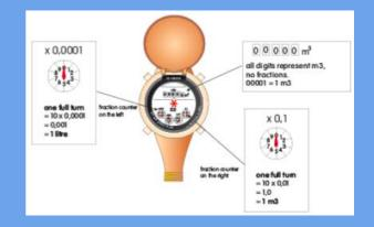
To regulate the flow, read the flow on the counter (no.1 from left is 1 l/min one full turn) adjust with regulating valve untill desired flow has been achieved.
