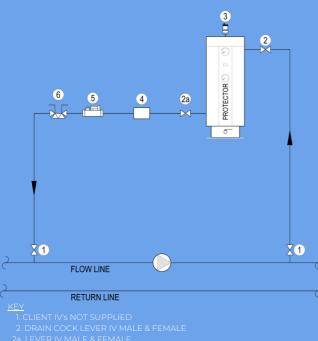
2a. LEVER IV MALE & FEMALE 3. 551 CALEFFI UNIT AIR VENT 4. MECHANICAL WATER METER
